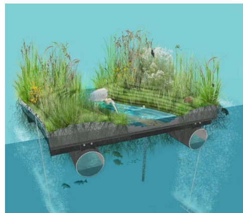
Figure 77. Cross-section Rendering of a Floating Wetland
