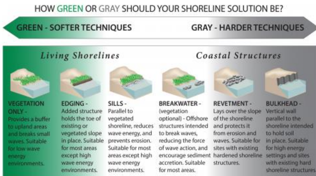
Figure 33. A Continuum of Green to Gray Shoreline Stabilization Techniques
